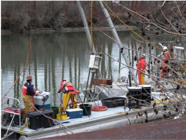
Vibracore sample being removed for processing
